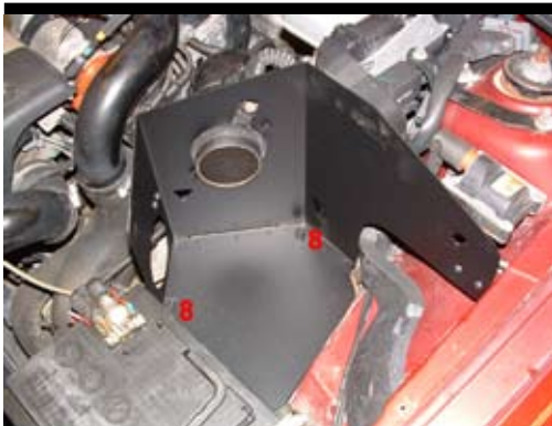
7. Assemble the heat shield. Press the shield downwards so it hits the lower original suspension attachment (8). Attach the bracket to the inner panel with the supplied screw.
