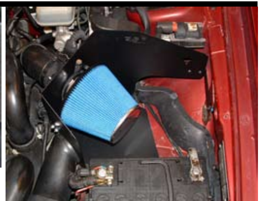
9. Attach the MAS to the heat shield. Use the supplied screws. Attach BSR airfilter and the inlet pipe.
