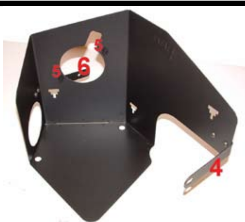
5. Shield preparation: Attach the bracket (4) and the clips (5). If the magnetic valve was screwed on, also mount the bracket (6).
