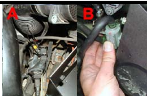
8. If the magnetic valve was screwed on, attach with the plastic ties (A), otherwise attach the magnetic valve directly to the pre-cut opening in the heat shield (B).
