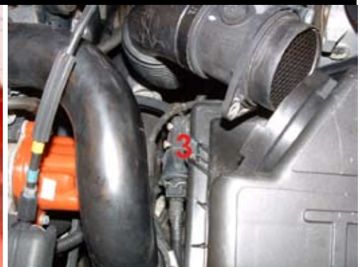
3. Remove the magnetic valve (3), and if fitted, the electrical harness from the air filter box.
