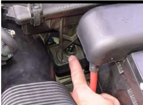
4. Remove the air filter box by pulling the right side upwards until it comes off the lower suspension attachment. Then pull sideways to remove it from the inner panel.
