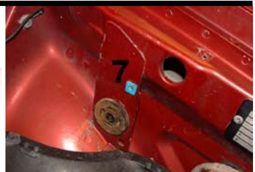
6. Attach the clip (7) to the inner panel.
