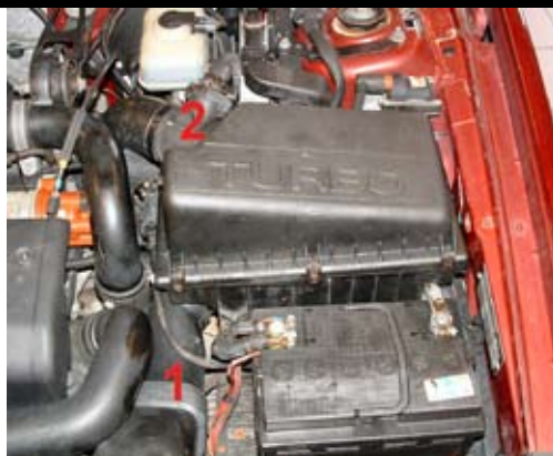
2. Remove inlet pipe (1). Remove MAS (2) (mass air sensor) from the air filter box.
