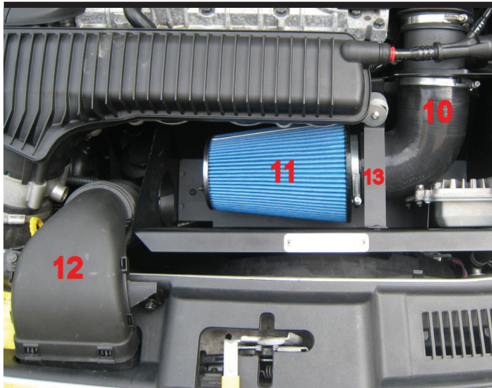
16. Assemble BSR air hose (10) and performance air filter(11). Assemble the rod(13) as picture. Lower the engine and assemble the bolts to the engine mounting. Assemble the inlet tubing (12) and reconnect the battery.
