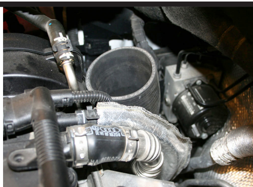
5. Assemble BSR intake hose pointing forward. Tighten with hose clamp 50-70mm.
