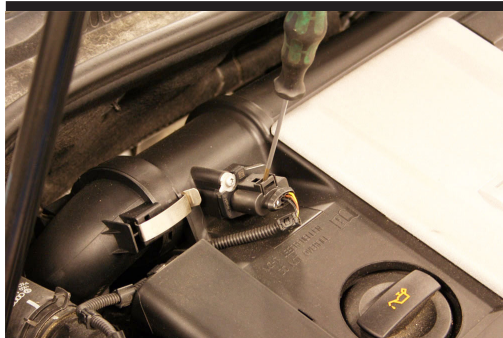
1. Disconnect the electrical plug from the mass air sensor (MAS). Use screwdriver as picture shown to remove.
